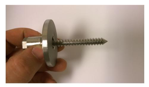
3) Using a stud-finder, locate a stud and spot drill it using a 3/16" drill bit (this is true for wood or steel/metal stud). Drive the assembled screw & flange in your hole and secure it using a 13mm wrench.
