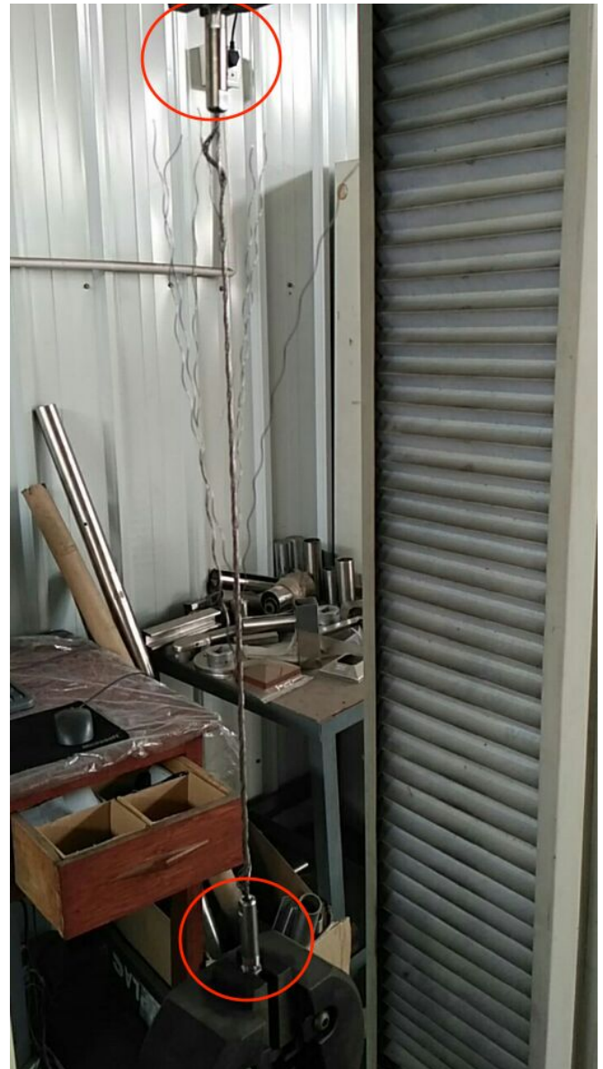
Pic.2 - The cable broke at a tension of 1924 lbs (8.56 kN) while the tensioners were still intact
