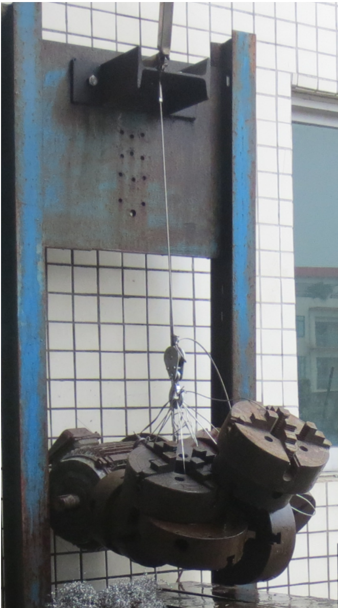
Pic.1 - Cable withstanding a load of 1200 lbs
